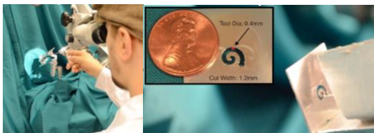
Fig. 1 Left: Microlaryngeal study setup. Right: Close up of the smallest spiral and the tool tip inserted into it.
